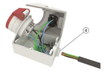
5. Screw the top part of the housing to the bottom part of the housing.
